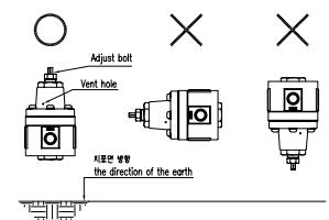
Fig. 2-1: The correct positions
